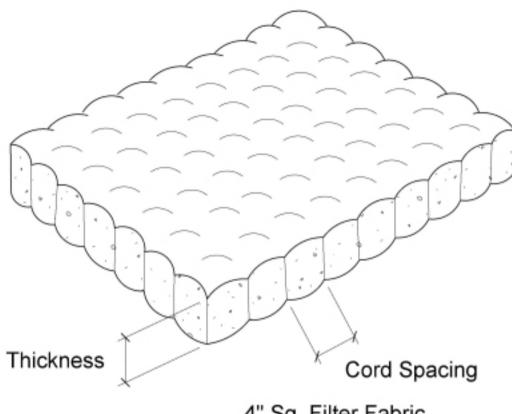
4" Sq. Filter Fabric placed and locked by Plastic Ring ————
